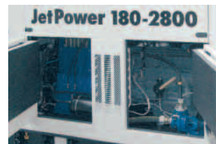
Optimum access due to many tiltable and removable protection hood components.
